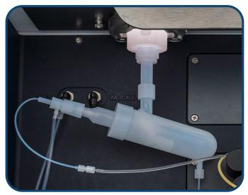
Fluorospray Sample Introduction Kit installed on Agilent 5900 ICP
