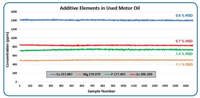
SampleSense Oil System 11+ hour stability run on iCAP PRO XPS for 4 additive elements
