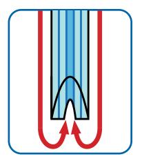
Closeup diagram of V-shaped tapered tip probe on SampleSense Oil system. The probe design allows the applied vacuum to efficiently remove sample droplets to eliminate contamination of other samples
