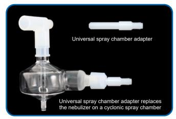
Universal spray chamber adaptor (P/N HG-USCA-01) used with hydrideICP operating in hydride-only mode.
