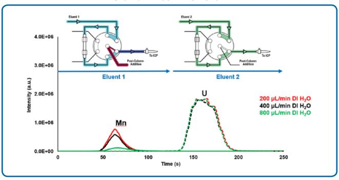
Separation of trace element impurities (e.g.,  $5 \mu g/mL$  Mn) from uranium matrix (1 vol. % U) using three post-column addition flow rates (200, 400, and 800  $\mu L/min$  DI water). The arrows depict the timing for switching the method from eluent 1 to eluent 2.
