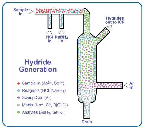
The patented design promotes HydridelCP's gas liquid separator is the smallest, highest performing and most stable on the market. The design promotes rapid mixing of sample and reagents, resulting in an efficient reaction and separation of hydride gases from sample liquids in a small volume.
