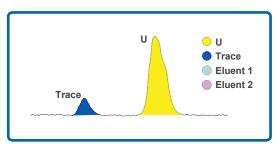
Illustration of the chromatographic separation of trace metals and uranium matrix using an UTEVA resin column.
