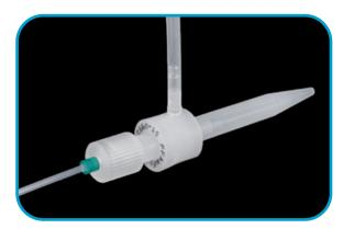
Sample capillary attached to PFA-ST MicroFlow nebulizer
