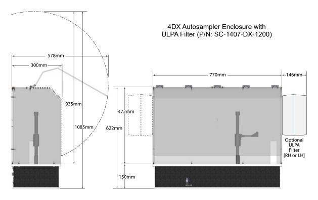
4DX autosampler with mobile stand and enclosure and ULPA filter, W x D X H: 77.0 x 34.6 x 127.3 cm
