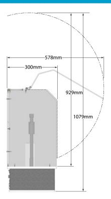
2DX Autosampler Enclosure with ULPA Filter (P/N: SC-1207-DX-1200)
