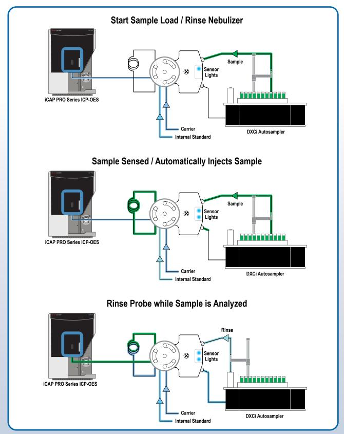
SampleSense FAST operation with iCAP PRO Series ICP-OES
