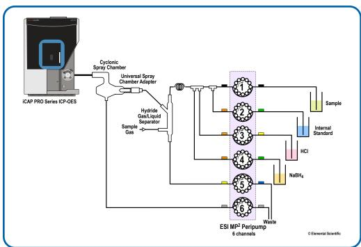
hydrideICP with internal standard system diagram
