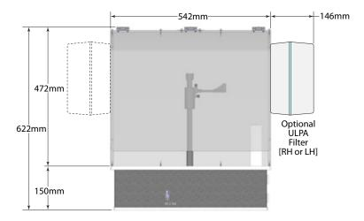
2DX autosampler with mobile stand and enclosure and ULPA Filter, W x D X H: 54.2 x 34.6 x 127.3 cm
