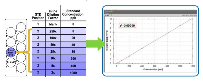
Autocalibration improves laboratory efficiency by eliminating the need for labor-intensive and error prone standard preparation. It reduces laboratory waste by reducing calibration vial, reagent, and standard waste. prep*FAST* autocalibration is particularly important for low concentration standards near the detection limit.
