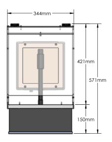
Micro DX autosampler and enclosure and ULPA Filter, W x D X H: 34.4 x 37.1 x 57.1 cm
