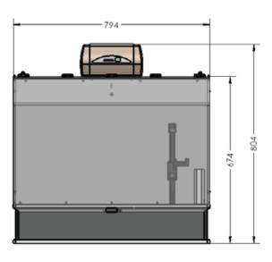
8DX benchtop autosampler with enclosure and ULPA filter, W x D x H: 79.4 x 54.8 x 80.4 cm
