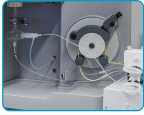
PFA MicroFlow OneTouch nebulizer with SampleSense prepFAST X on iCAP PRO Series ICP-OES
