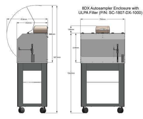
8DX autosampler and ULPA filter, W x D X H: 79.4 x 55.2 x 154.2 cm
