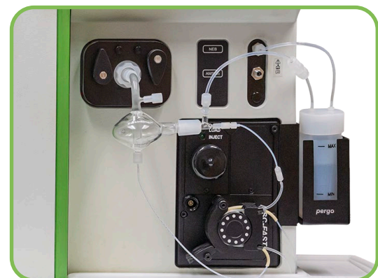
pergo 2000 systems mount onto existing NexION 1000/2000 pumps as well as FAST and prepFAST DXi modules
